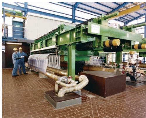
Figure 5. The modern hydrochloric acid electrolyzer plant for chlorine production installed at Brunsbüttel, Germany (photo Bayer MaterialScience AG)
